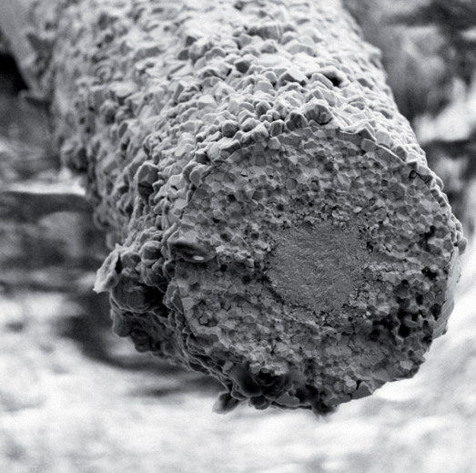
▲ Hydrogen induced embrittlement of tungsten
