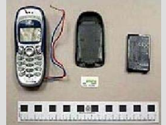
Top: Mobile phone detonator from Madrid bombings. Below: SIM card subjected to 450°C, average desk height temperature in a house fire.
